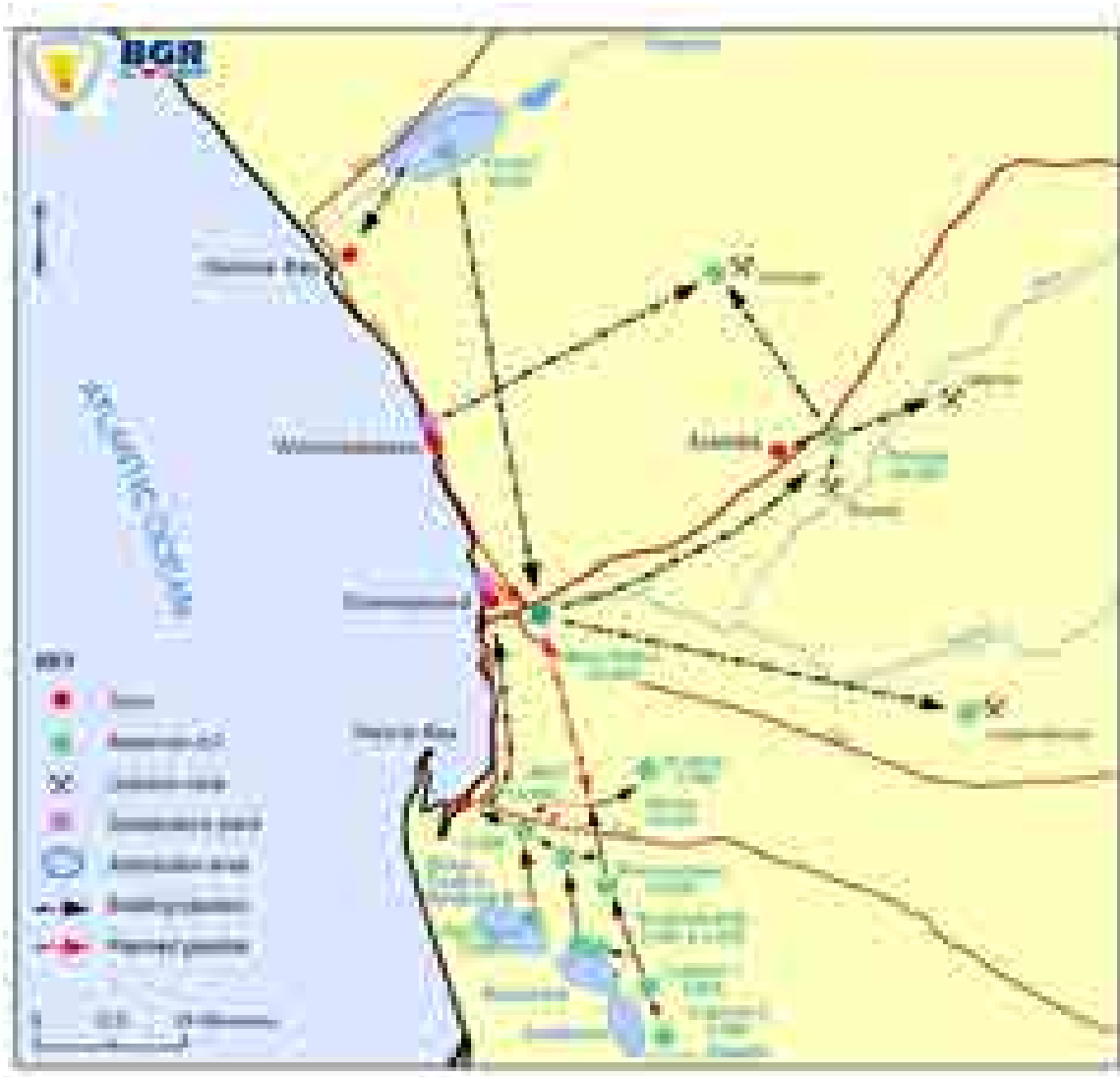
Figure 7.4.4: Layout of the existing Central Namib Area Bulk Water Supply System and proposed new developments. (Source: NamWater)
